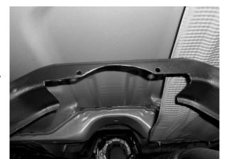
to the close proximity of fuel tank to this area, we DO NOT recommend using a flame-cutting torch or plasma cutter when performing these operations. Also, excess heat can easily damage the frame and other adjoining components
