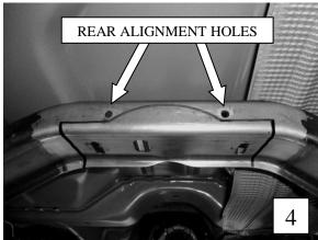
**Warning!** Check the backside of the crossmember to be sure that all lines, electrical wiring, control cables and other components are cleared from this area to avoid damaging them in the following steps. Be sure to wear proper safety protection when using power tools! **DO NOT** create sparks near flammable or explosive materials. **Due**
